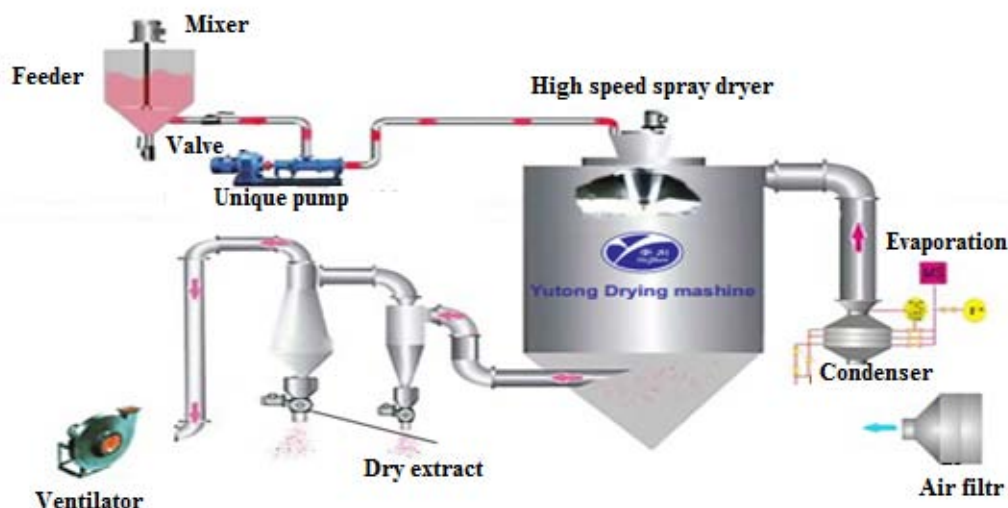
Fig. 2: Spray dryer "LPG-15 HIGH SPEED SPRAY DRYER"
