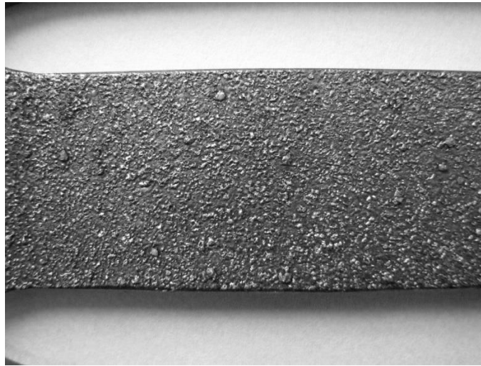
Figure 3. The appearance of the sample surface strengthened by alloy T15K6
