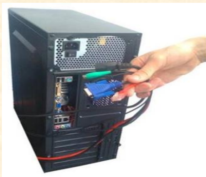
2-rasm. Barcha tashqi kabellarni ajratib olish.
