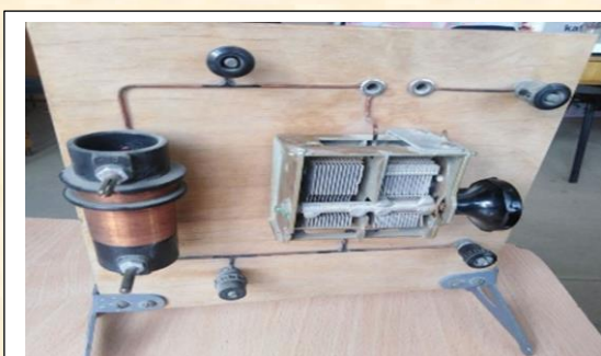
4-rasm. O'zgaruvchan sig'imli kondensator.
