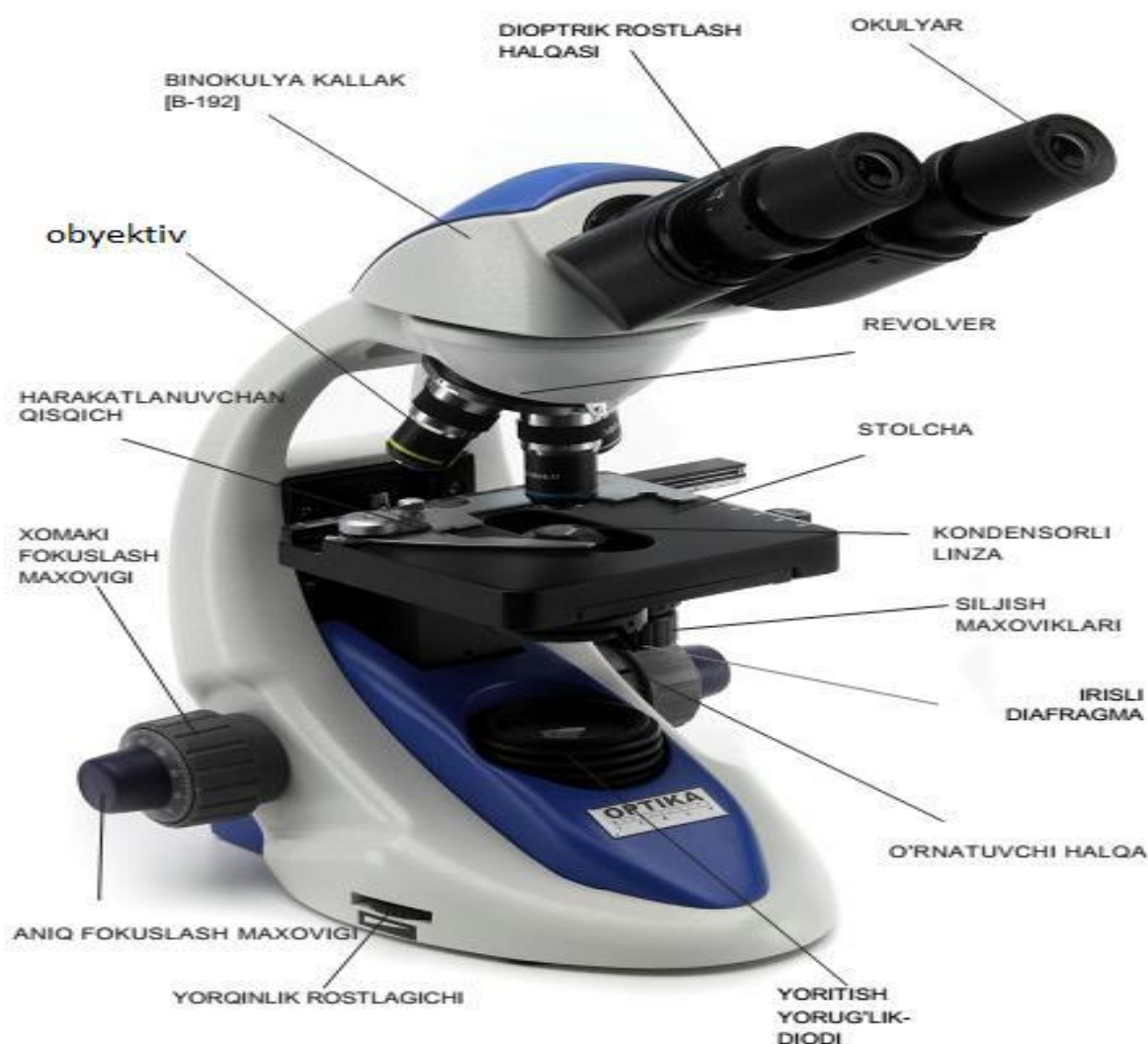
2-rasm. OPTIKA ITALY B-191 rusumli binokulyar mikroskop tuzilishi
