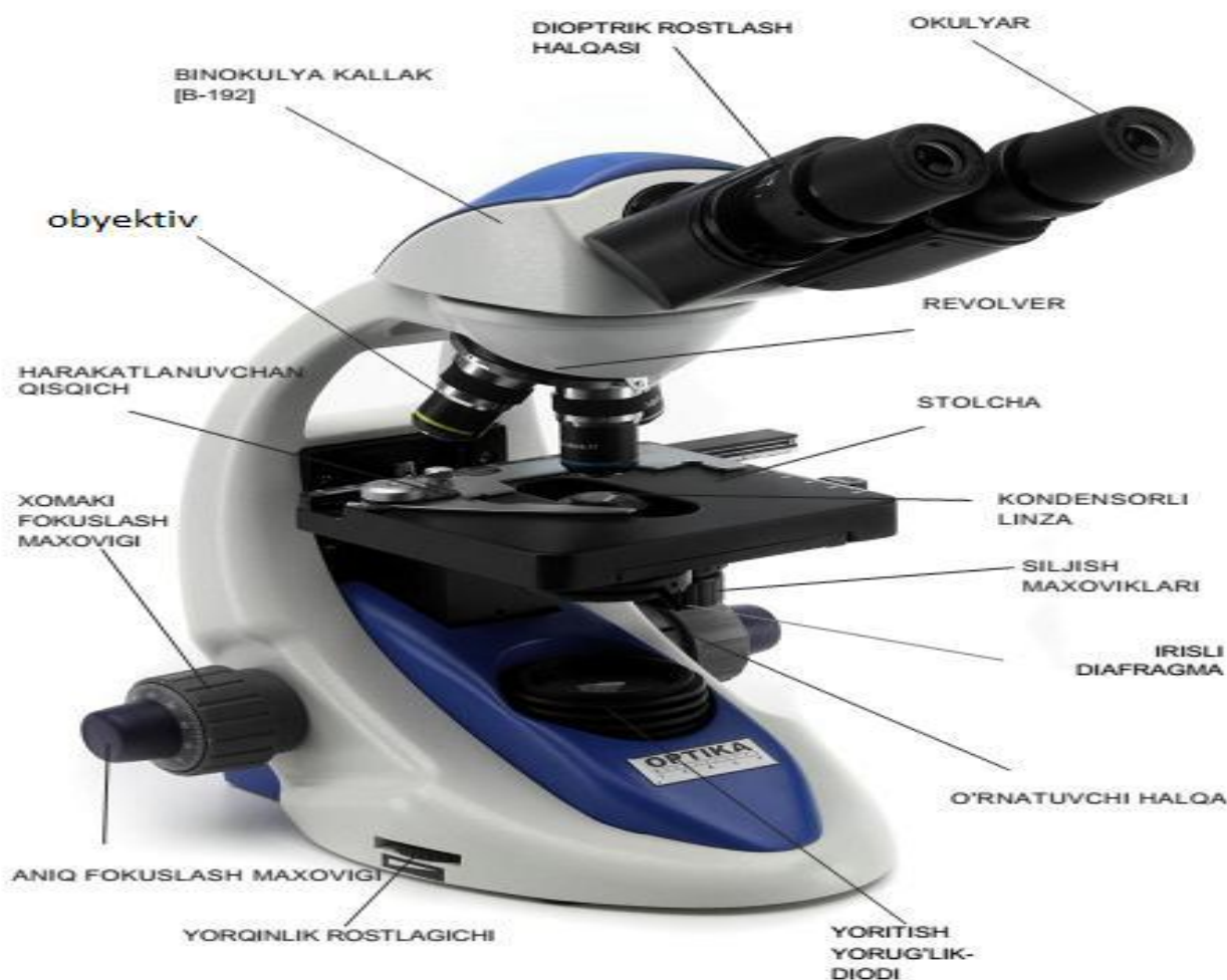
14-rasm. OPTIKA ITALY B-191 rusumli binokulyar mikroskop tuzilishi
