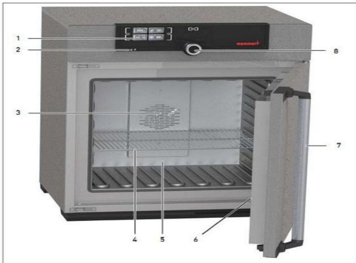
5-rasm. Memmert-IF 110- rusumli termostatning tuzilishi.
